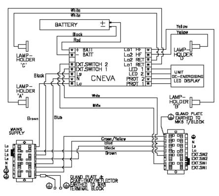
Typical wiring diagram shows circuit with inhibition terminals installed for information only, some models may differ. I-PRSE-10 IOM PRSE BI EM LT Issue 07 01/01/2021 3
